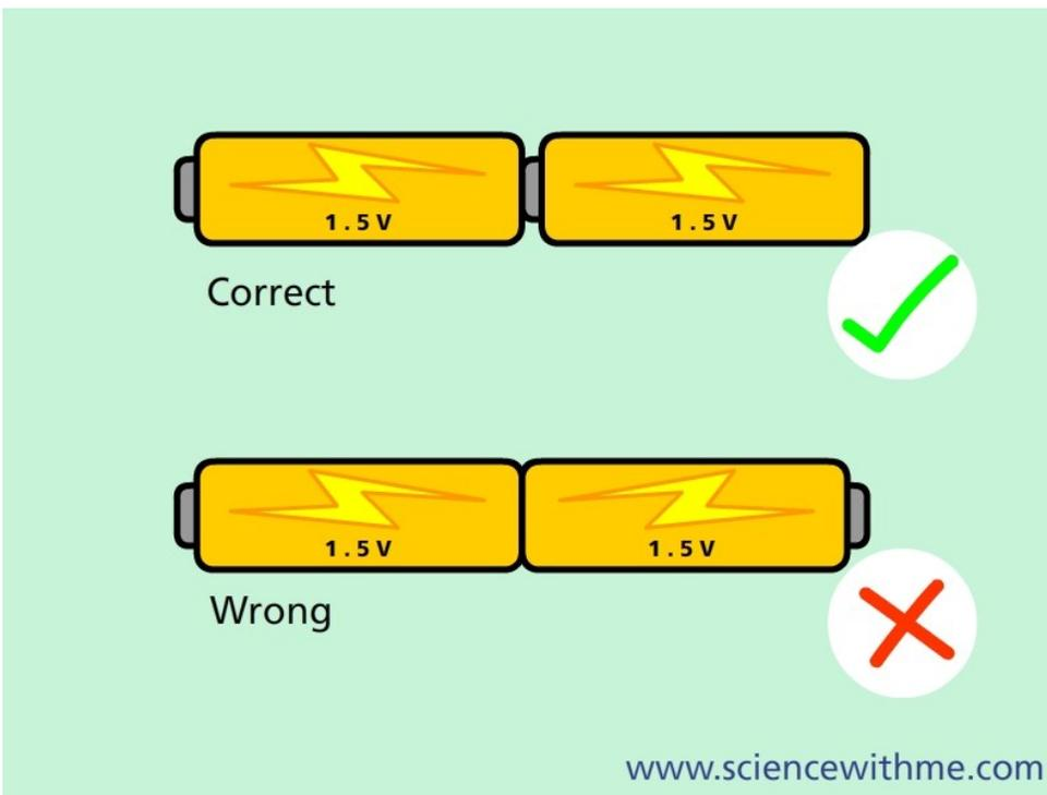
Adding more cells in a line (in series) will make the bulb burn brighter.
